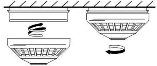
If you have difficulty locating onto the base, it could be that the ring has been moved to the locked position while away from the base.
