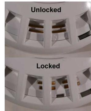
View into rear with base removed. Ensure that cabling does not press against the internal boards when installed on the base.
