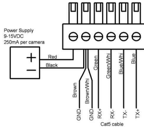
Wiring for Networked configurations
