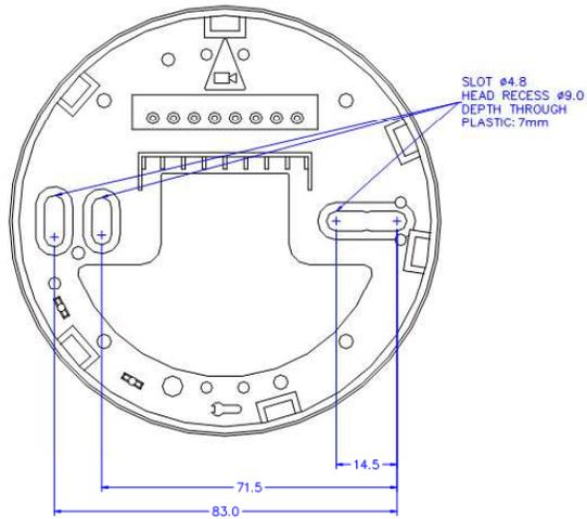
CEILING MOUNT POSITION USING MOUNTING BAR
